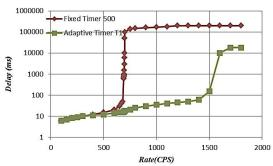
FIGURE 5. Throughput with adaptive and fixed timer T<sub>1</sub>
