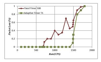
FIGURE 9. Packet Loss with adaptive and fixed timer T<sub>1</sub>
